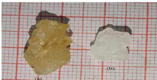
Figure.1: Grown crystals of (a) pure and (b) magnesium chloride doped L-histidinetetrafluoroborate (L-HTFB)
